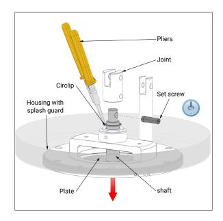
Tighten the plate B between soft jaws in a vice.
