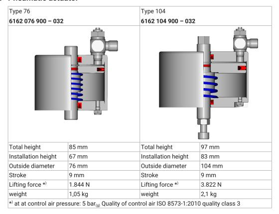
The selection of the actuator size can be made according to the following table:
